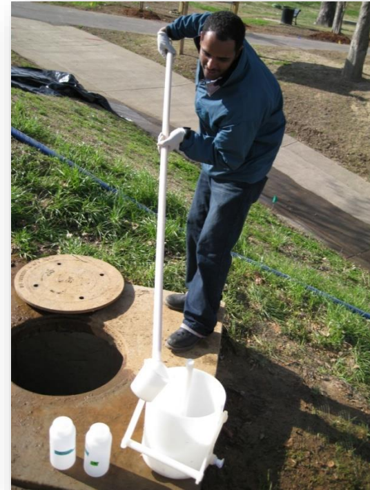
Grab sampling in outlet chamber
