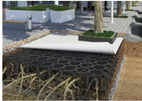
Structural Soil System
